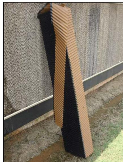
Figure 6. Weak pad glue joints.
