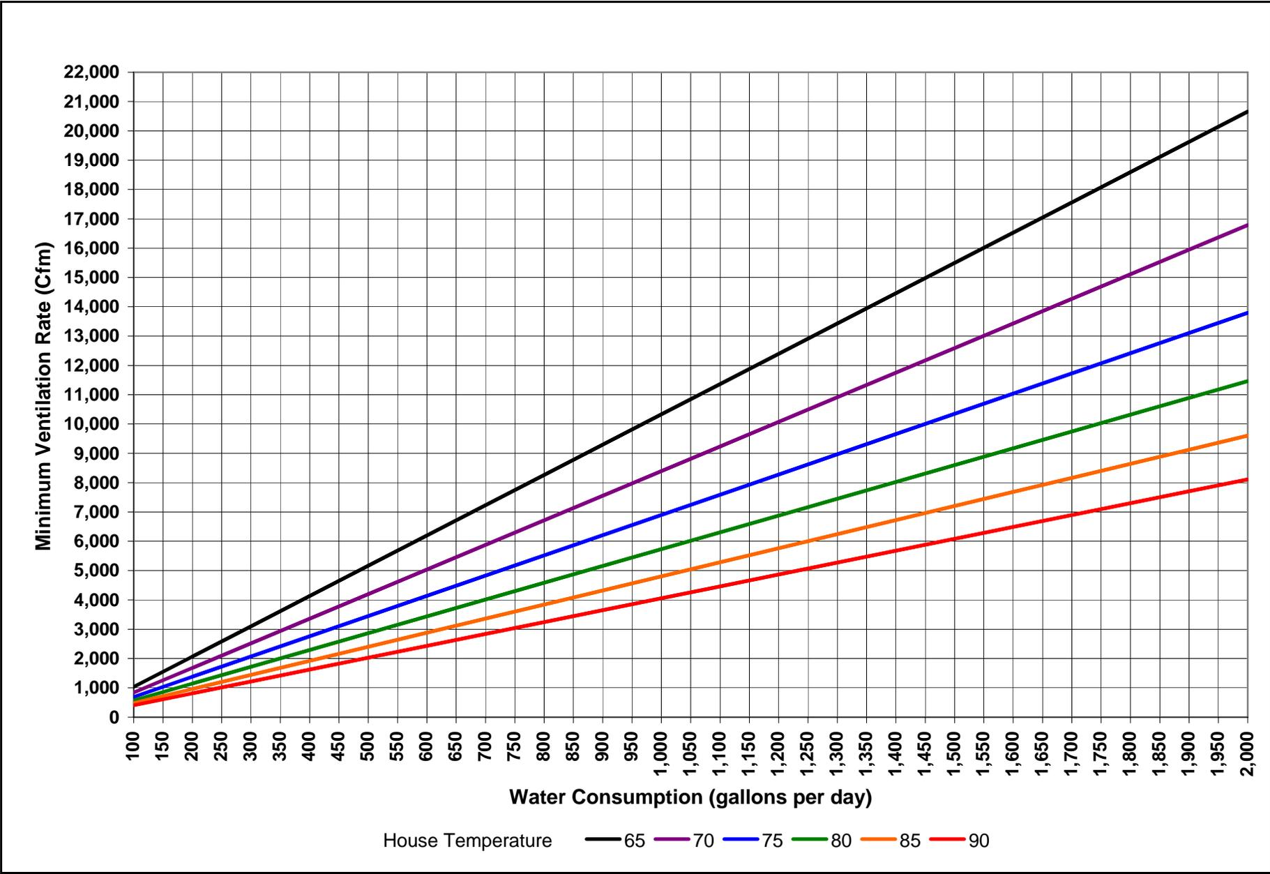
Figure 2. Minimum ventilation rates required to manage house moisture based on bird water usage and inside temperature.
