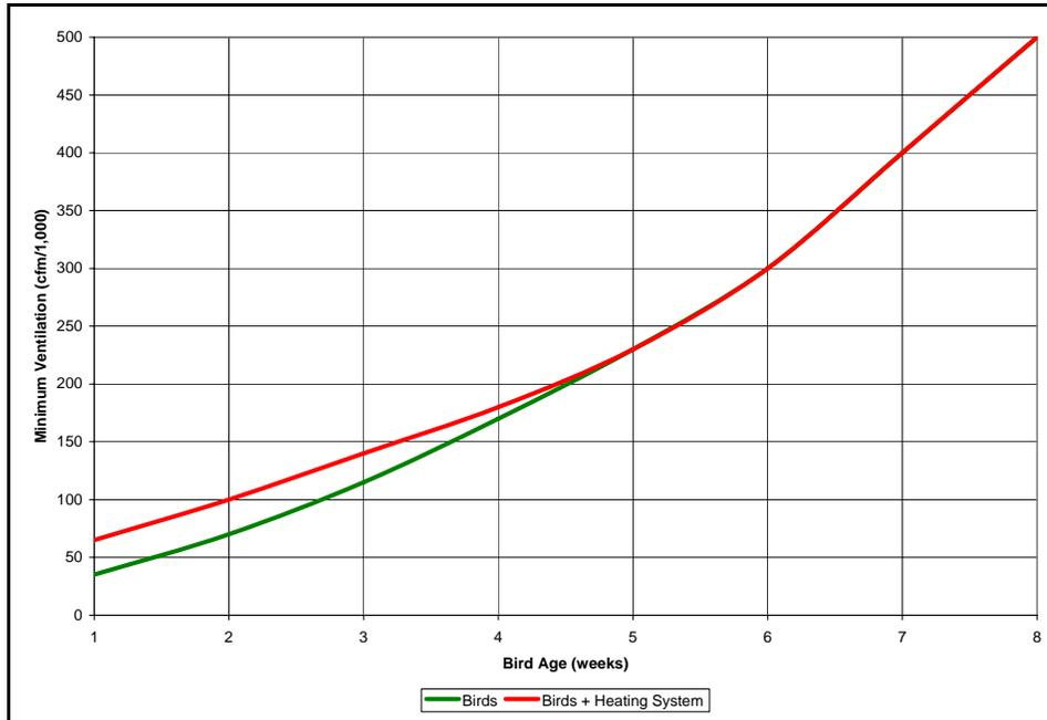
Figure 1. Minimum ventilation rates to control carbon dioxide.
