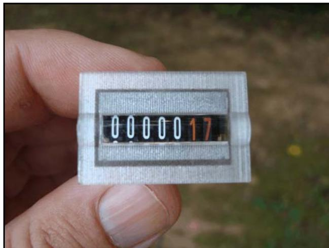
Figure 4. Optional mechanical Kw\*hr display.
