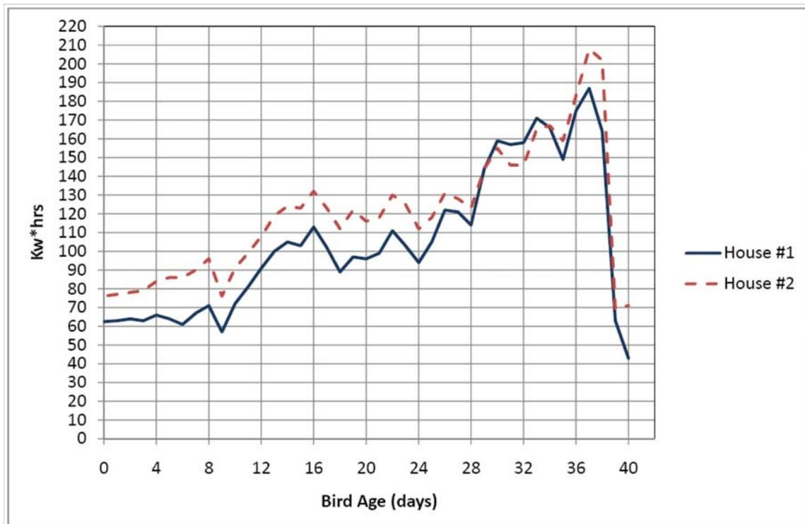
Figure 5. Daily power usage for two tunnel-ventilated broiler houses.
