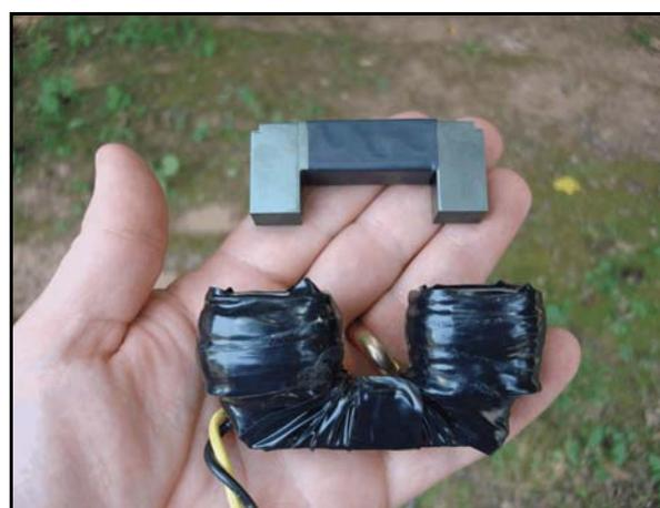
Figure 3. Split-core current transformer
