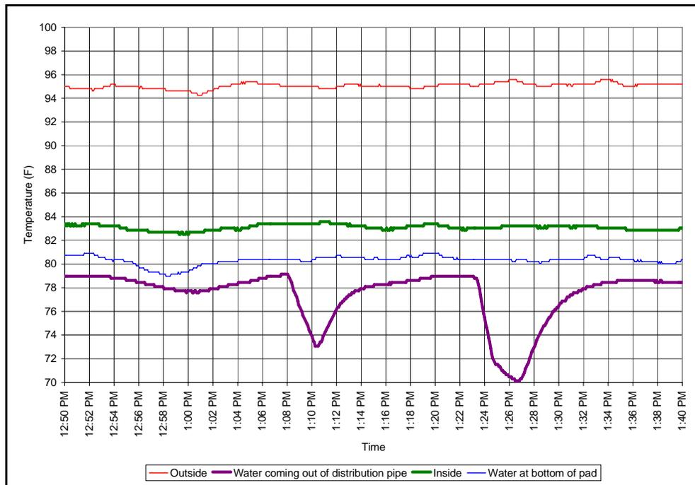
Figure 2. The effects of adding ice to a six-inch-pad system on a hot day.
